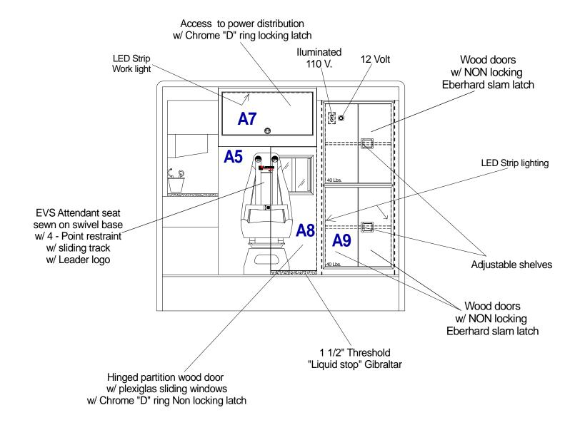
Type 3 LE\_94 / 148 94" X 148" Module on Ford E350 138" WB chassis, 72" Headroom Curbside 3/8" Recessed Plexsiglas doors w/ 02 outlet Chrome "D" ring latches Digital 15 min. Cargo Net Blue Academy Re-stocking Timer (Black) LED Strip independence Lighting Upholstery and Fillers S / S Antimicrobial Grab Bar 圍 Electric door lock switch (wired to OEM) IMMI 4 PT **A10** Per4Max Seat belts Blue Reflective 3M Diamond Grade LED Step Well light **Sharps Container Trash Container**
